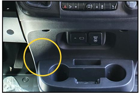
1. The grey connector on vehicle side might be found directly inside the radio tunnel, or below the plastic cover for the FIAT wireless Qi charger. In this later case, the connector might be taped along the FIAT harness: just remove the tape and connect it to the supplied harness.
